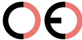
False CE Mark (too far)
